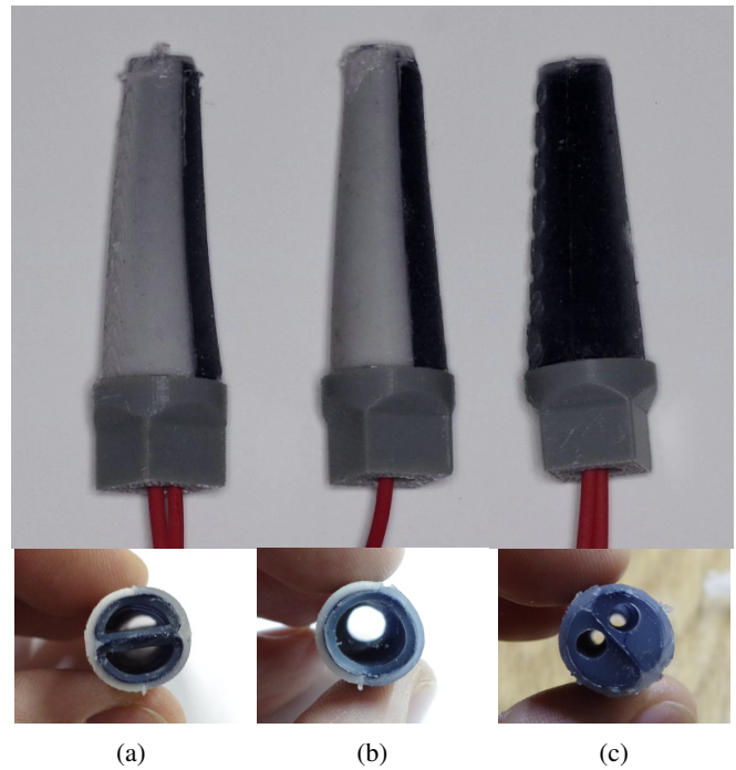
Fig. 7: Tested actuators (a) - proposed actuator, (b) - single DOF actuator, (c) - actuator based on unsymmetrical actuation. All the actuators have same dimensions.
