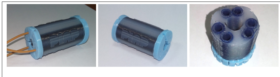
Fig. 1: Single module design. On the left: module; on the right: module cross-section, reinforced actuation chambers and central channel visible
