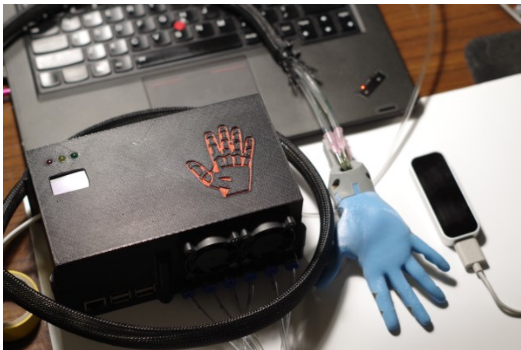
Figure 5.49: The pressure control box along with soft hand and Leap motion controller.
