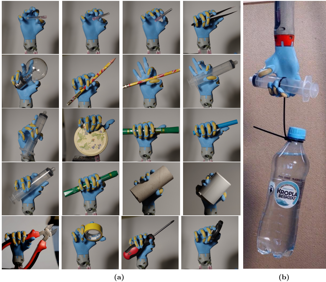
Figure 5.18: Grasping tests, (a) various grasping postures picked from Kapandji score test [154], images from [142], (b) an exemplary load applied to the hand. Total mass of the object and syringe 550g. In both cases all the actuators are connected to the same pressure source.
